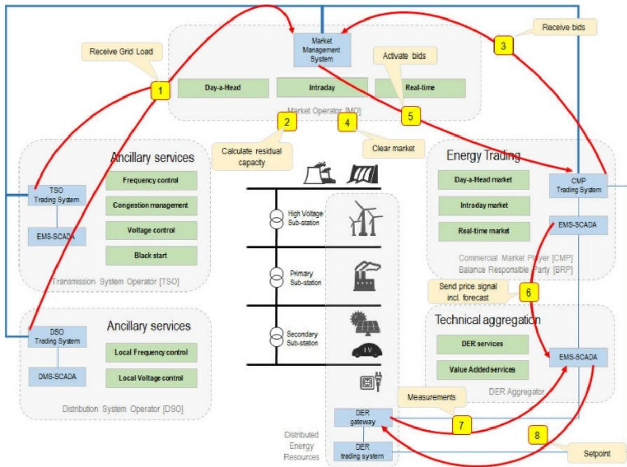
Figure 4. SmartNet ICT reference model applied to the Danish pilot.
