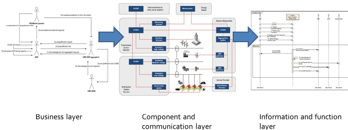
**Figure 1. Transition from business actors into system components and interfaces, as presenting exchanged information objects with sequence diagrams.**
